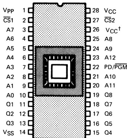
†V<sub>CC</sub> may be connected to pin 26 for 24-pin ROM compatibility.
